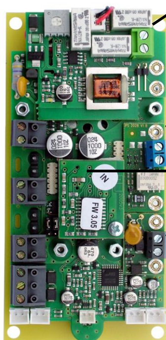
2N® SingleTalk with removed cover for illustration, equipped with all extending module types
