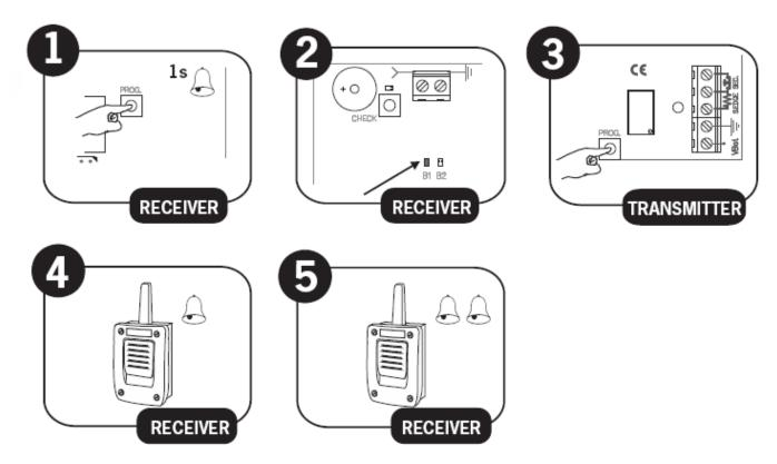
If 10 seconds pass without programming a transmitter, the receiver will exit the programming mode. If when programming a transmitter the receiver's memory is full then it will emit 7 beeps of 0.5 sec and exit the programming mode.
