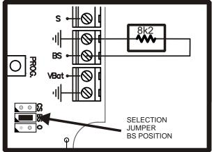
$\begin{array}{lll} \text{SEdge Detection} & \text{Ok}\Omega - 5,8k\Omega \\ \text{SEdge Ok} & 7k\Omega - 9k\Omega \\ \text{SEdge Open} & 11k\Omega - \infty \\ \end{array}$
