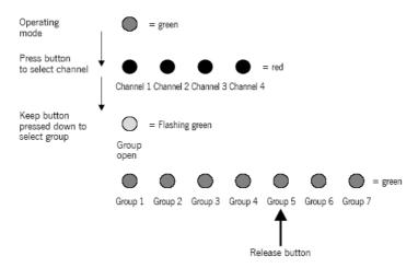
Channel: This allows for the channel to be sent to the receiver to be selected. Group: This allows for the installation of more independently enabled doors (to a total of 22).
