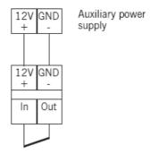
Wiring diagram for the installation of more than one activator in series (maximum 4) and avoiding interference between them. To do so, the OUT synch. signal must be connected to the IN synch. signal of the following activator.
