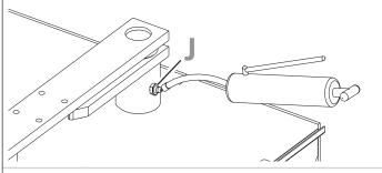
Lubricate the wing device through the lubricating nipple (J) until grease escapes on both sides (grease DIN 51502 KP 2 N - K 2 K-20).
