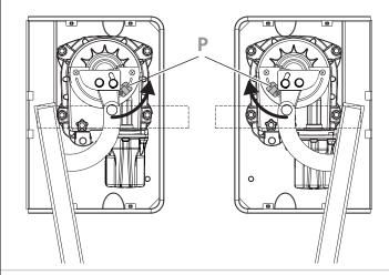
Attach the reference point sensor (P) so that the rotatable arm moves over the reference point sensor every time that the gate
