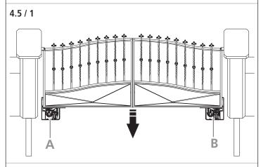
• Allocate the motors to the gate sides so that the motors are facing the direction of opening.
