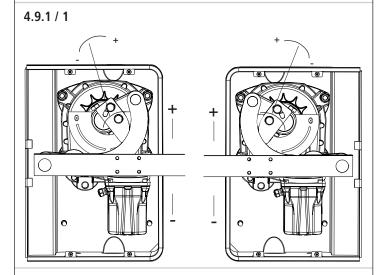
• Set the limit stop with the aid of the the fixing screws (O).
