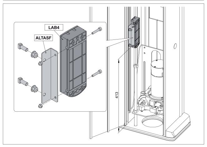
Install the ALTASF photocell support and the LAB4 photocell as shown in the figure. NOTE: check that the external photocell is correctly aligned with the internal photocell.
