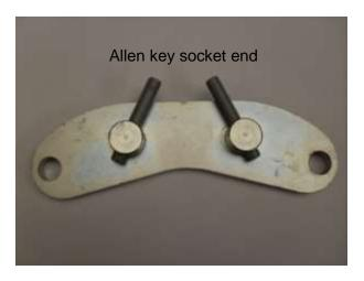
Screw the 60 x 8mm threaded rod into the turrets on the underside of the linkage arm as shown above.
