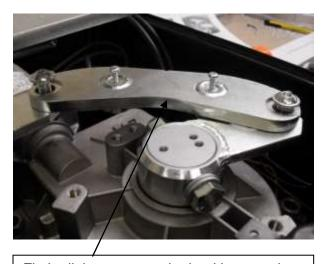
Fit the linkage arm to the load lever and the gearbox rotation arm. Grease the threads and fit the domed Allen head screws
