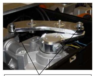
With the 19mm spanner hold the linkage locking nut on the underside of the load lever and the gearbox rotation arm.
