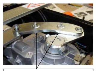
Adjust the VRO & VRC so that the gate stops in the required open and closed position.
