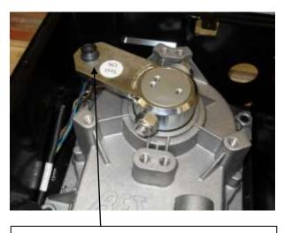
Grease and Insert the linkage locking nut into the gearbox rotation lever from the underside as shown
