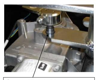
Grease and Insert the linkage locking nut into the load lever arm from the underside as shown above
