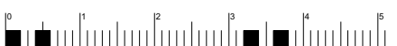
Programming and waiting Indicates the programming mode or the waiting status of the external user
