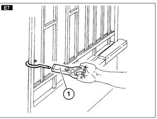
In the event of a power failure, release the operator in order to open the gate by hand.
