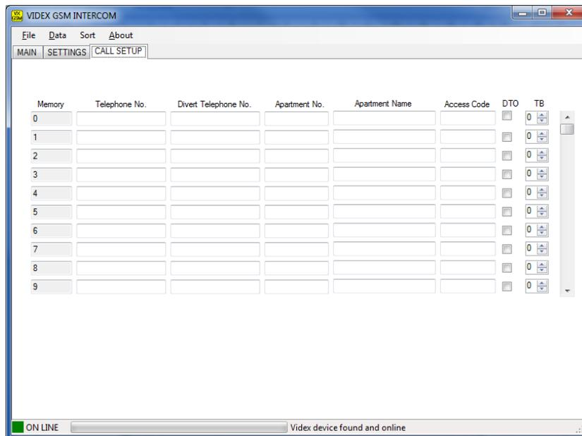
From the call setup page it is possible to assign up to 2 telephone numbers to each of the 1000 available locations. The divert telephone number will be used if the call is busy or not answered and will divert to this number after the divert time has elapsed. If no divert number is stored, the first number will continue to ring until the call times out.
