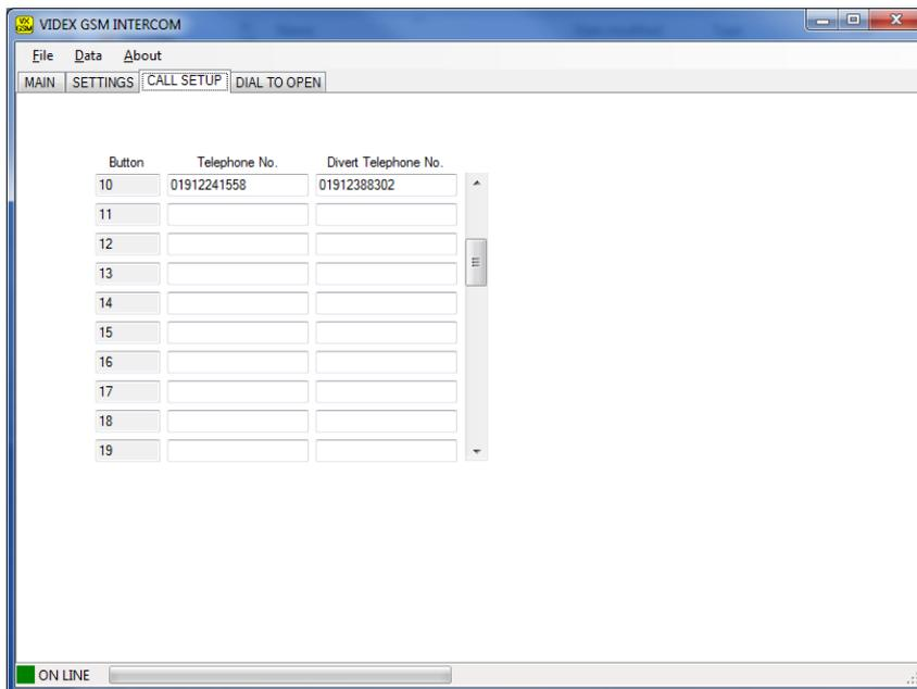
From the call setup page it is possible to assign up to 2 telephone numbers to each of the 50 available call buttons. The divert telephone number will be used if the call is busy or not answered and will divert to this number after the divert time has elapsed. If no divert number is stored, the first number will continue to ring until the call times out.
