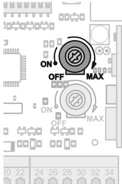
If required, you can set how much warning you want using potentiometer 1. While the warning time is running, the external warning light flashes. When set all the way to the left, this function is deactivated.
