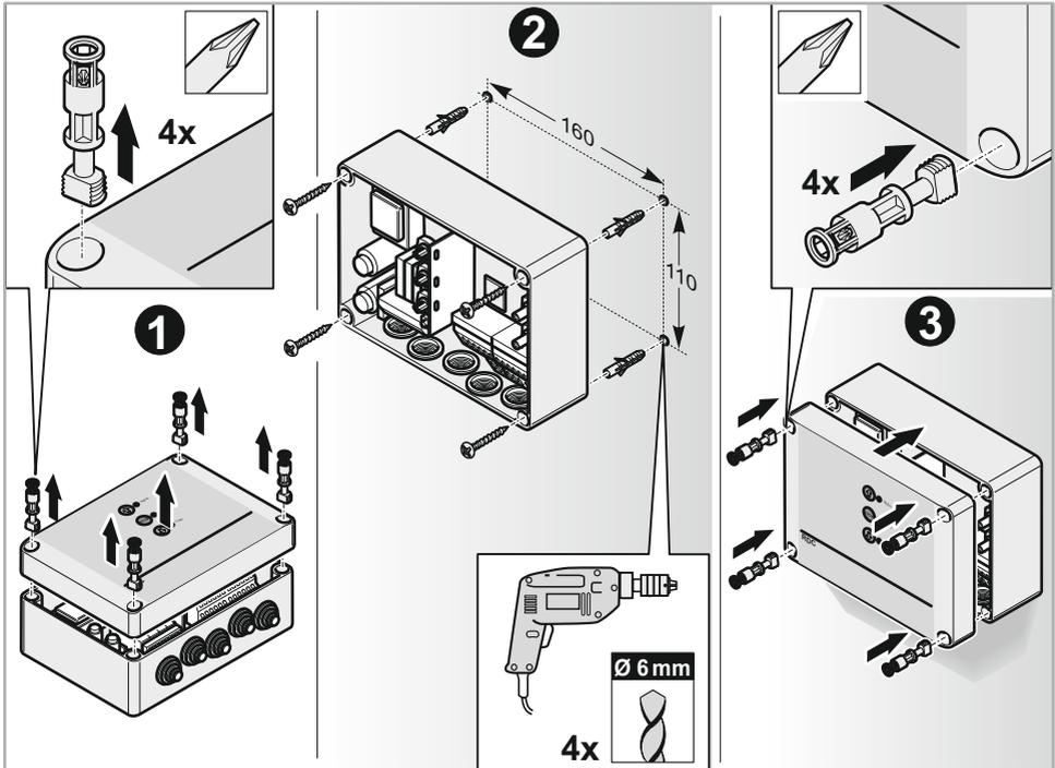
Install the housing upright on an even surface, with the cable conduits facing downwards.
