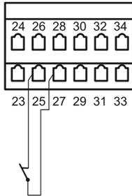
When pressed, the EMERGENCY OFF switch stops the operator immediately and terminates all control unit functions (including dead man operation).
