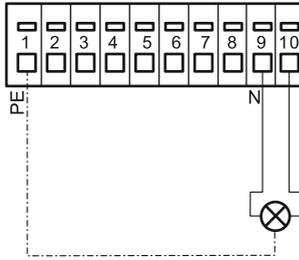
The warning light gets its power supply from the control unit (AC 230 V, max. 80 W). It has two flashing patterns:
