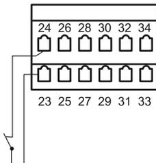
The arrester is installed in the door operator and can be connected to the control unit. If it is, the control unit detects when the arrester kicks in and blocks all control unit functions.
