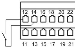
The pre-limit switch is mounted on the bottom of the door frame, max. 5 cm from the floor. After the pre-limit switch is activated (the door overruns the position when closing) the safety contact strip must be activated within 2 seconds or the operator goes into reverse; the door opens.
