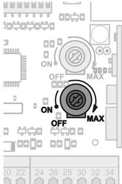
Automatic closing is activated when potentiometer 2 is switched on (turned clockwise). The potentiometer is switched off by factory default (set all the way to the left). Turn it clockwise to set the stay open time. The maximum stay open time is approx. 120 seconds. During the stay open time, LED1 (Status) flashes once intermittently.
