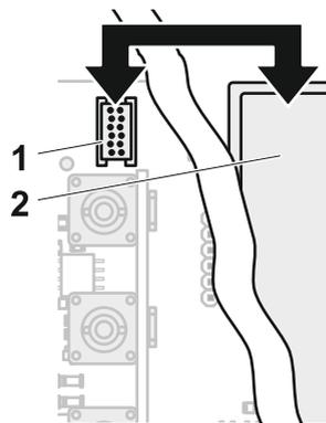
A TorMinal (2) can be connected to connection (1). A TorMinal is a device for reading out and adjusting factory-set control unit values. TorMinal may only be operated by an expert with the relevant skills.
