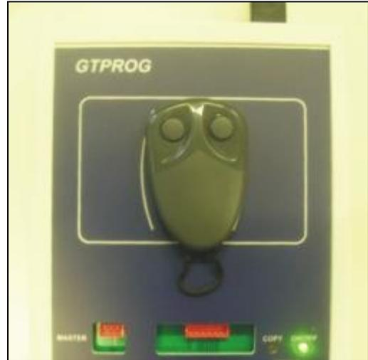
If a GTSYSTEM terminal is used, after pressing "OK" place the transmitter to program under the programming interface, press and then release the interface button. The transmitter LED flashes and the interface LED lights up steady.
