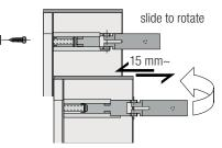
Snap the cover onto the hinges. Close it and secure it using the supplied screws. After the settings and adjustments, fasten the cover using the supplied screws.
