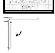
5. Once the procedure is over, the display will show **[Travel calibr OK]** for a few seconds.
