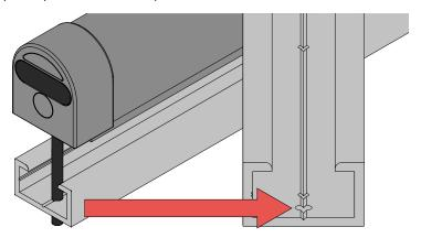
3. Drill an additional 8mm hole in the desired location to draw any cables through the alu carrier and frame of gate/door.
