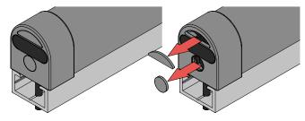
7. Finally ensure that water drains from the end caps have been removed as illustrated (for vertical installations remove only the lower water drain (for horizontal installations remove water drains from both ends of the safety edge) !WARNING! failure to remove water drains from the safety edge will invalidate any warranty.
