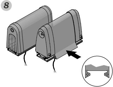
**!NOTE: Pulling or pushing the safety edge into the aluminium C-profile can cause damage to the contact edge and should be avoided at all costs !**
