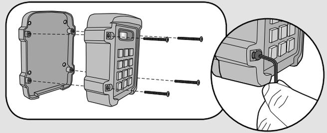
Mount the Keypad onto the back panel with screws. Tighten screws with Allen wrench.
