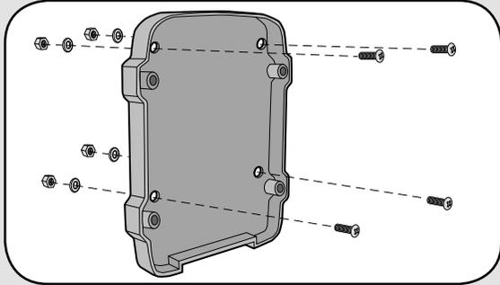
Choose mounting location for Keypad. Remove the back panel and attach it to a solid surface or post.
