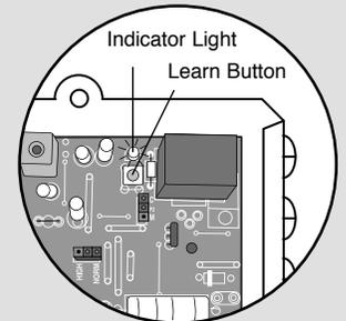
**Step 2:** Press and release the Learn button on the receiver. The Indicator Light will light for 30 seconds indicating that receiver is in Learn Mode.
