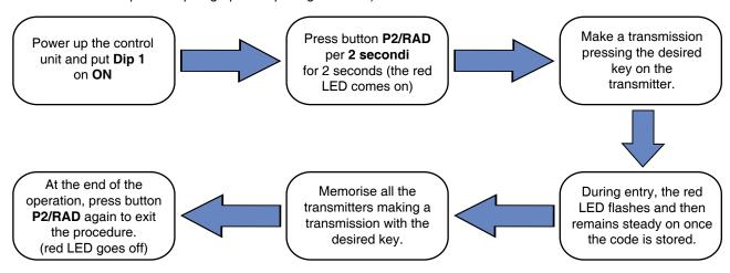
① The programming procedures are exited automatically in any case 10 seconds after the last transmission.
