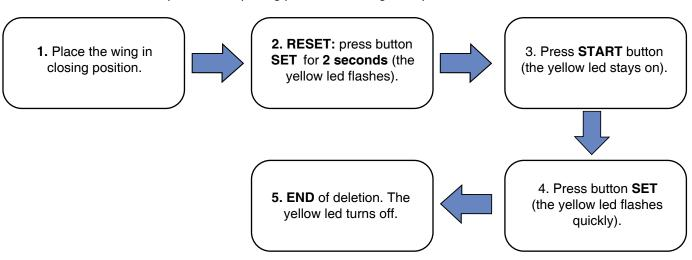
After the deletion, it will be possible to activate the pedestrian opening only by wire, and the size of the opening will be total on the wing.
