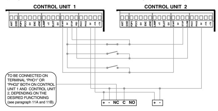
① Since there are two different receivers, there is the possibility that the radio signal could not be received simultaneously.
