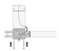
With the reduction gear rotated, insert the motor and cap, and insert the cable.
