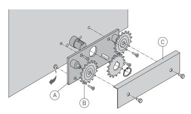
N.B.: Install the chain traction kit before securing the gearmotor to the base plate.
