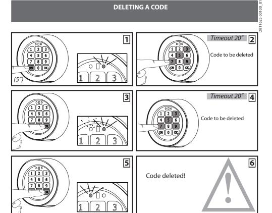
**WARNING:** if you delete the last code, you will no longer be able to activate the relevant control unit. To restore operation, you must perform the total deletion procedure to erase all codes and repeat installation from the beginning. It is advisable to delete the codes of channels that are not associated with anything (e.g. code 2222, 3333, 4444, 0000 etc. when using a single control unit).
