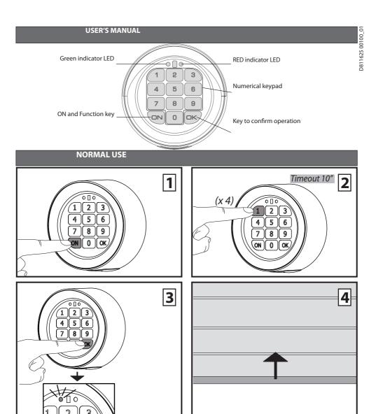
**WARNING:** T-BOX will lockout after 3 consecutive incorrect codes are entered and will not accept further codes for 90 seconds. If another incorrect code is entered, T-BOX will lockout at the first attempt.
